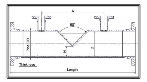
Installation Requirement : down to 5 x D for Up-stream and 2 x D for Down-stream
